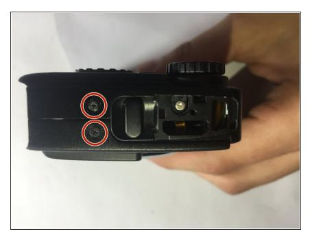
There are two screws to remove on the right side of the camera, which are marked in the photo. These screws are
