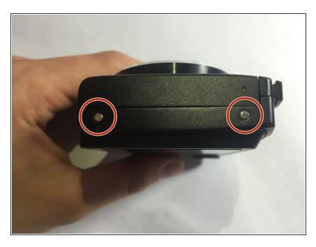
There are two screws in the left side of the camera, which are marked in the photo. These screws are
