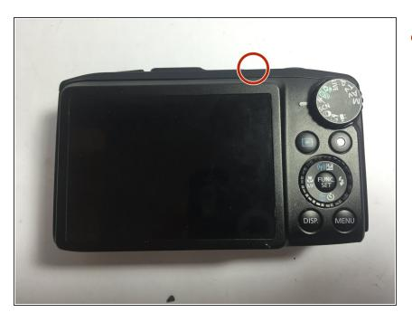
Turn off the camera by holding the ON/OFF on the top of the camera.
