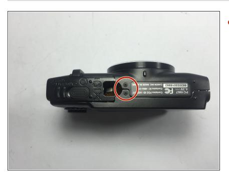
Finally, there are two screws on the bottom that need to be removed.
