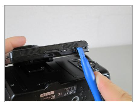
Pry the casing apart using your plastic opening tool. Begin by prying at the hole where you removed the screw and continue along the seam.
