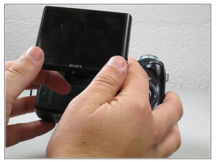
• Extend the LCD screen away from the camera to access the screws on the back of its housing.
