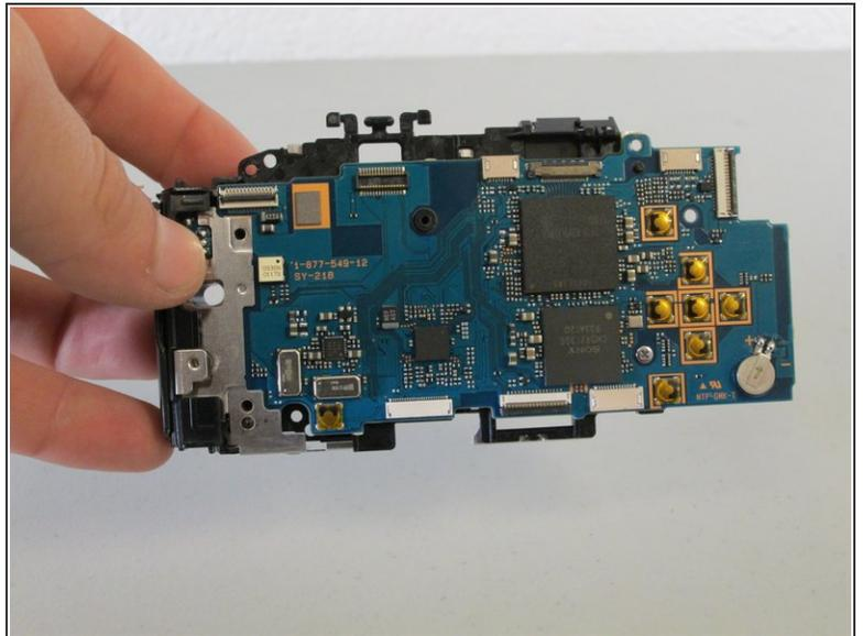
**!** If you feel resistance from the board, double check all screws and cables have been removed to avoid damage.
