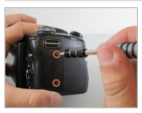
Remove the two #00 4.0 mm Phillips screws shown on the side of the camera.
