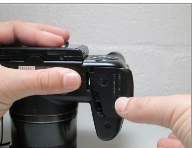
Close the battery cover by pushing the cover inwards and sliding it to the left to allow more maneuverability when disassembling other parts of the camera.
