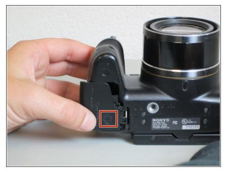
Push down and away from the camera to the left on the indicated indentation in the battery cover. The compartment should slide open as shown.
