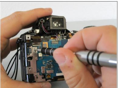
Detach the metal bracket from the enclosure by removing the two #00 4.0 mm Phillips screws.
