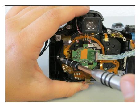
Unscrew the #00 6.0 mm Phillips screw on the left side of the lens.
