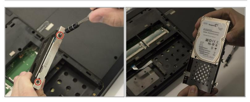
Unscrew two 3mm Phillips #0 screws to remove the casing on the hard drive.
