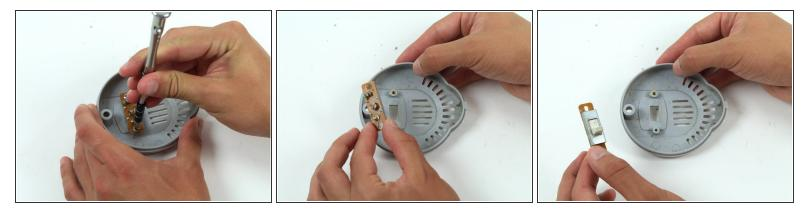
• Unscrew the switch from the back panel and remove it.
