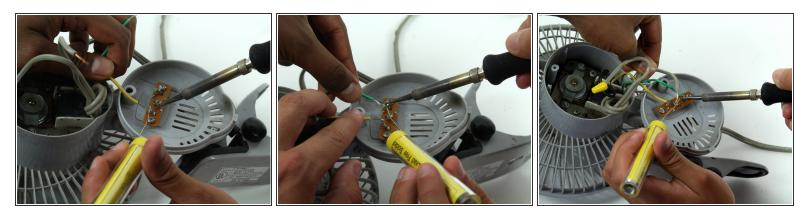
• After replacing the switch, resolder the gray power cord, the green wire, and the yellow wire.
