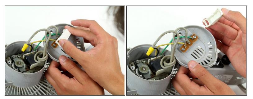
• Remove the plastic cover on the switch by pulling it apart from the the back panel.
