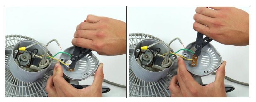
• Cut the green and yellow wire as close to the switch connection as possible.
