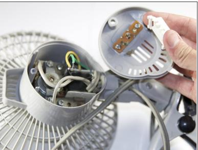
Remove the plastic cover on the switch by pulling it apart from the back panel.
