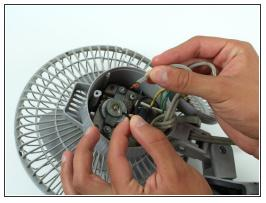
Unscrew the yellow cap that connects the black wire and the gray power cord wire. Then, unwind
