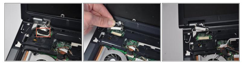
Unplug the black cable with rectangular white plastic head from the motherboard. It is located at the top left of the motherboard, directly below the left hinge.
