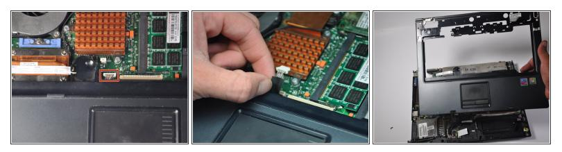
Unplug the white cord connecting the mousepad to the motherboard from the motherboard, and pull off the entire plastic panel.
