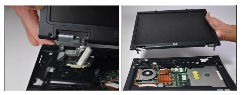
• Pull the monitor directly upwards from where it lay. The two metal hinges should easily slide out of their holes and the monitor will be disconnected from the motherboard.
