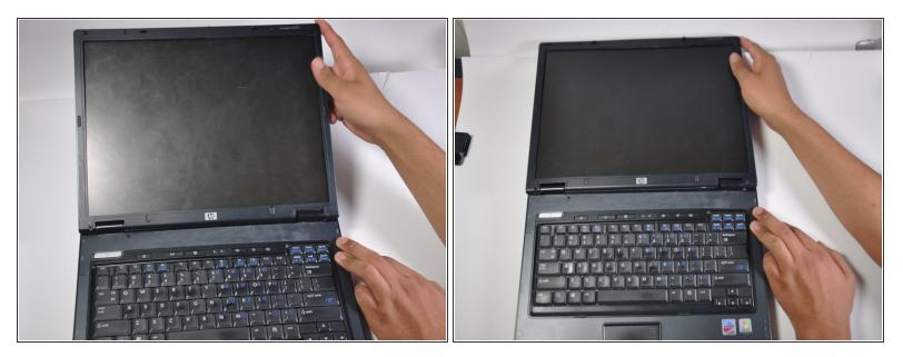
• Open up the laptop so that the screen is facing towards you. Push the monitor back until it is flat, parallel to the keyboard.
