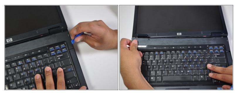
Using the iFixit opening tool, remove the plastic panel located between the keyboard and monitor.
