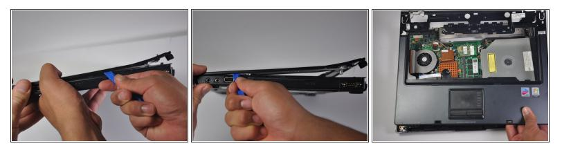
• Using the iFixit opening tool, pry the black plastic panel (with mousepad) off of the motherboard.
