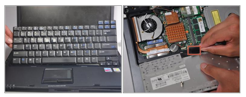
Flip the keyboard away from the monitor, rotating it so that the keys are face down on the mousepad. Remove the black cord at the bottom of the keyboard that connects it to the motherboard. The keyboard is now free and can be removed.
