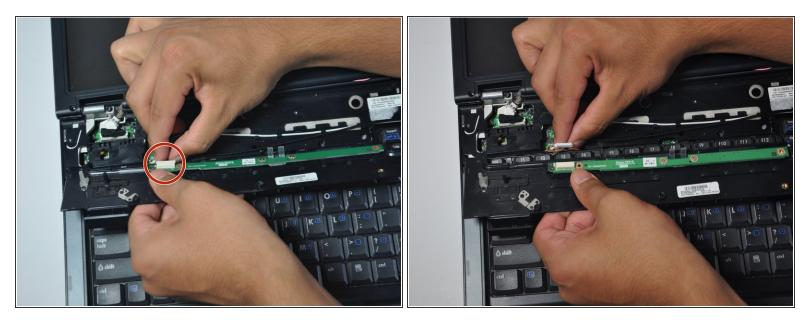
• Remove the white cable attached to the just-removed plastic panel from the motherboard.
