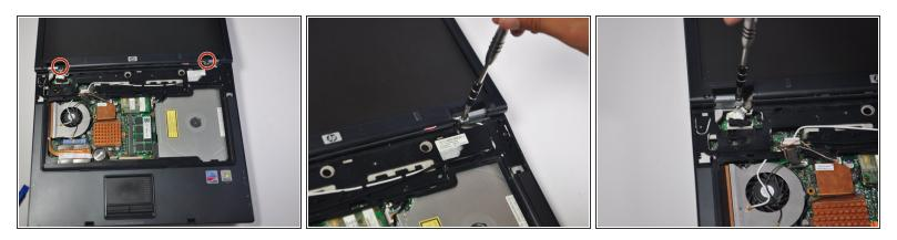
Remove the two 9.8mm 3.0 flathead screws. There is one at each of the hinges.
