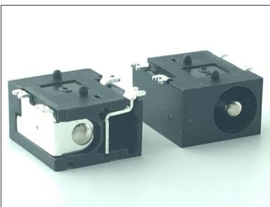
The new charge port will need to be soldered to the logic board. For an exact match use Digi-Key part number CP-018HPJCT-ND
