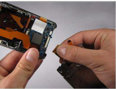
Disconnect the large ribbon-wire by pulling on the large ribbon-wire where it connects to the motherboard.
