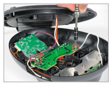
Remove the two 7.5 mm Phillips #2 screws holding in the motherboard
