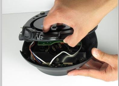
Remove the four 12 mm Phillips #2 screws surrounding the base then lift the bottom half of the base to expose the circuit boards inside the device.
