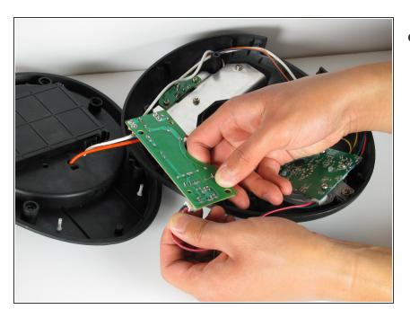
Lift the motherboard out of the device
