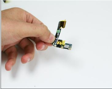
• Use a pair of tweezers to remove the headphone jack/micro USB board.
