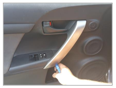
• Using plastic pry tool. Pry silver cover from handle.
