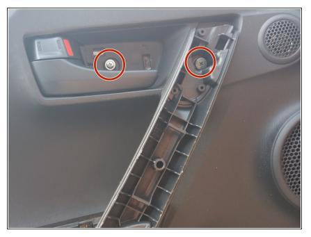
Remove the #4 25mm screw and the #2 25mm screw on panel with a standard Phillips Screwdriver.
