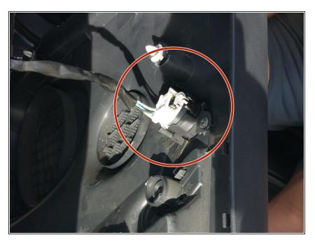
• Once door panel is free, remember to remove header from the tweeter in upper right hand corner of panel.
