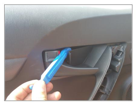
• Using pry tool. Pry off plastic plate in section of door lock or pull handle.
