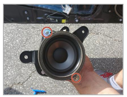
Remove speaker from bracket by unscrewing the two #2 12mm screws using a Phillips head screwdriver.
