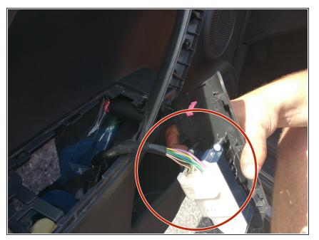
Un-attach white header(connector) from control panel. Push side tab on side of white connector if a little stuck.
