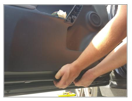
Pry Off Full Door Panel starting at bottom and working up the side, pulling fairly hard waiting. Clicking noises are a good sign the door panel is unlocking.
