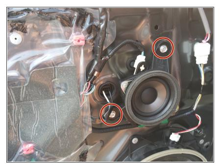
Remove bracket from door by unscrewing the two 14 mm nuts pictured here connected to the speaker unit.
