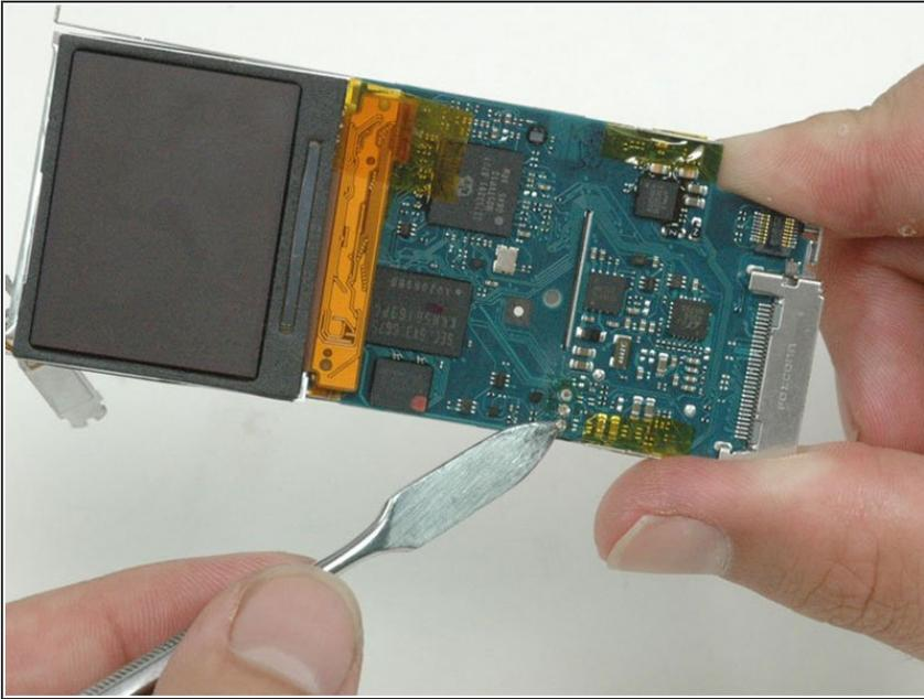
**⚠** Be careful not to scrape the metal rings surrounding the connectors off the logic board. If you accidentally scrape these off, you won't be able to reconnect the replacement battery.
