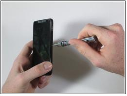
Remove the six 4mm T3 Torx screws. There are 3 on each side of the device.
