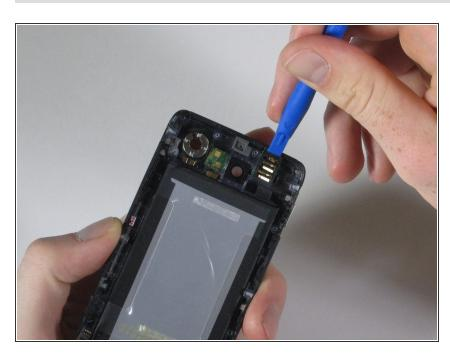
• Wedge a small plastic opening tool between the top edge of the headphone jack and the rear assembly casing. There is adhesive securing the headphone jack so you may need to use a decent amount of force to pry away the headphone jack from its clear plastic casing. To reassemble your device, follow these instructions in reverse order.
