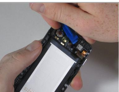
Wedge the plastic opening tool between the front-facing camera's casing and the rear assembly.
