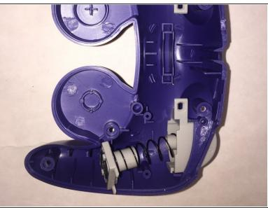
To remove the left and right bumpers from the bottom of the controller, pull up on the square base that keeps the button in place and then pull the button through the shell.
