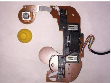
Once the control panel is removed from the controller the c-stick can be easily, but carefully, removed.
