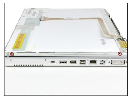
Remove the two small 3 mm black Phillips screws from the port side of the display.
