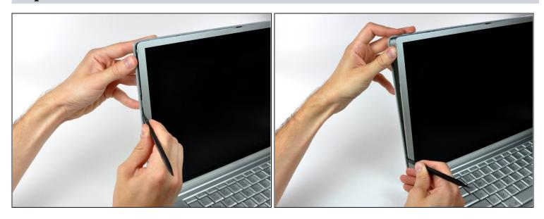
• Now that the top edge is released, use a spudger to completely release the clips along the left edge of the display.
