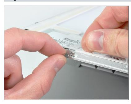
Remove the small magnet near the top left corner of the display, making sure to mark its orientation before removal.
