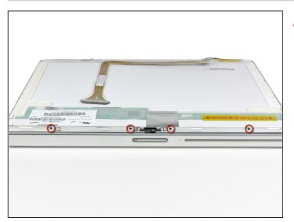
Remove the four small 3 mm black Phillips screws along the top edge of the display.
