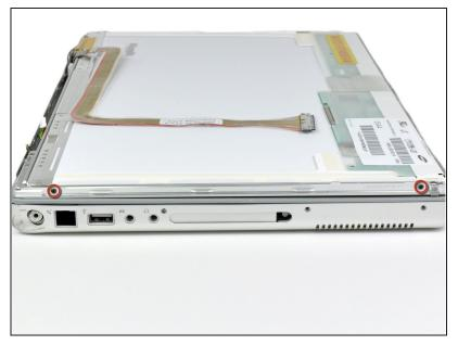
Remove the two small 3 mm black Phillips screws along DC-In side of the display.
