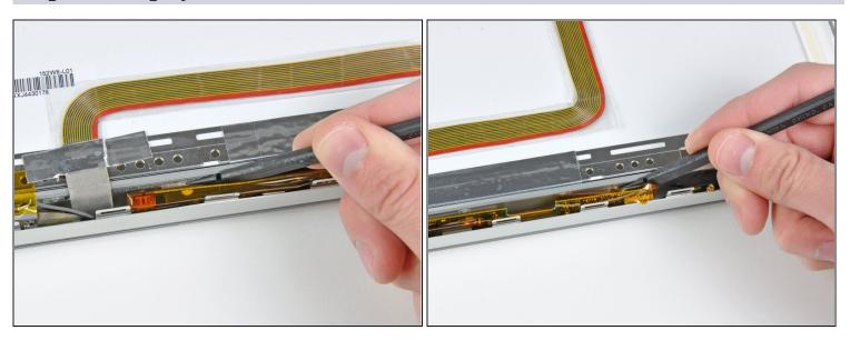
(i) If necessary, use the flat end of a spudger to peel the tape securing both ends of the display inverter to the clutch cover.
