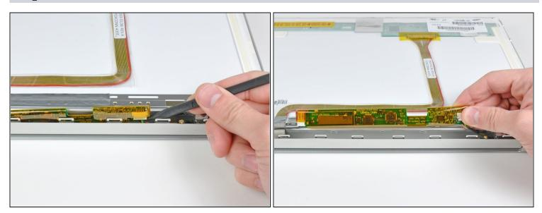
⚠ The inverter is an extremely thin circuit board that is very delicate and easily cracked. Take care when handling.
