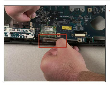
Push out the back of the casing by the VGA connector to remove the motherboard.
