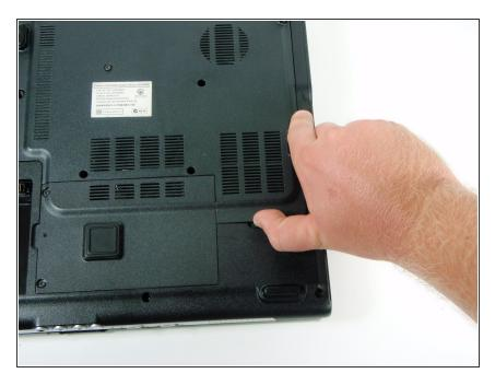
Lift up and remove the RAM and CPU cover.
