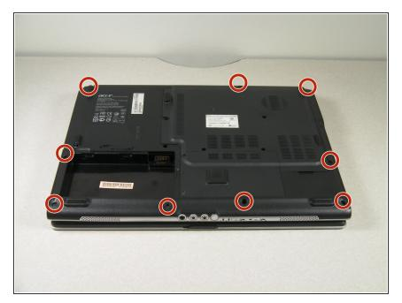
Remove the nine screws from the back edges of the laptop.
