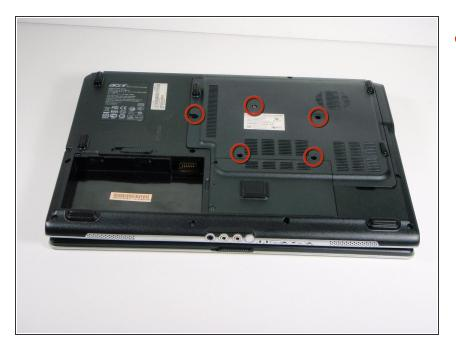
Locate and remove the 5 screws that secure the panel over the RAM and CPU cover on the upper right hand side. These can be found in the center towards the corner opposite the battery compartment.
