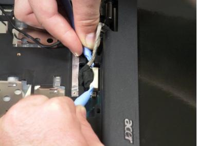
Detach the white rectangle located on the motherboard at the end of the wire connected to the LCD screen.
