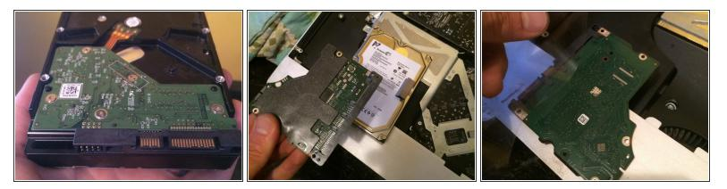
Pretty simple guide here . UNSCREW the logic board PCB from the ORIGINAL hard drive from the iMac 2009/2010/2011+ Hard dive for step 1:
