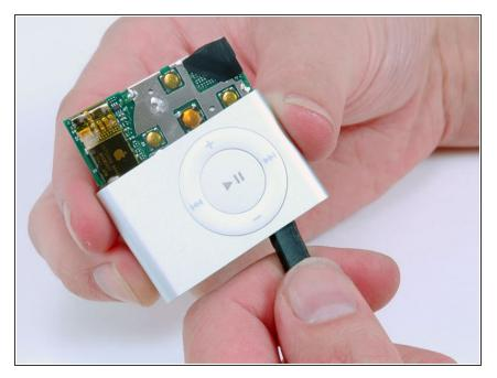
Use a spudger to push the logic board through the case and out of the Shuffle.
