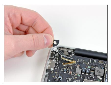
Remove the small rubber gasket from the corner of the upper case near the display data cable.
