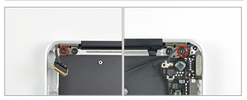
Remove the outer 4.9 mm T8 Torx screw securing each display hinge to the upper case (two screws total).
