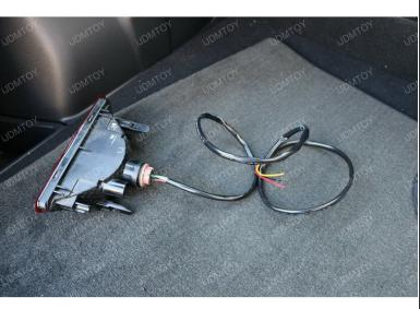
Install the socket into the housing. It should fit very tightly. If it is a little bit loose, you can apply some silicone glue around the outer corners of the socket to create a tighter seal.
