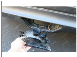
Remove the screws holding the bulbless rear reflector in place and then remove the entire rear reflector assembly.
