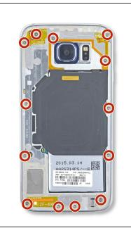
Remove the thirteen 3.5mm Phillips #00 screws securing the midframe to the phone.
