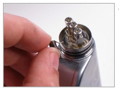
• Gently remove the burnt coil from the positive and negative screws.
