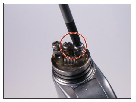
Using a Phillips screwdriver, gently turn clockwise to tighten down the positive and negative screws onto the coil.
