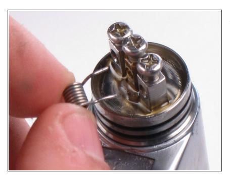
Place the new coil into the holes underneath the positive and negative screws.
