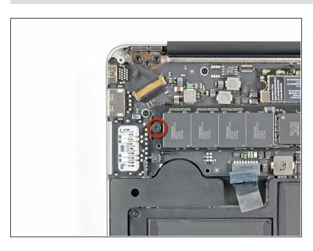
Remove the single 2.9 mm T5 Torx screw securing the SSD to the logic board.
