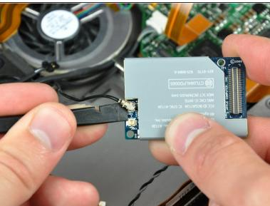
Use the flat end of a spudger to pry both antenna connectors up off the AirPort/Bluetooth board.
