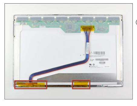
if present, remove the pieces of tape stuck to the lower edge of the LCD.
