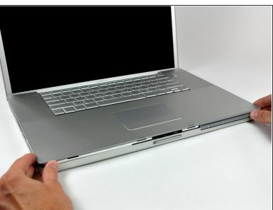
Starting near the display, lift the upper case straight up off the lower case, minding any cables that may get caught.
