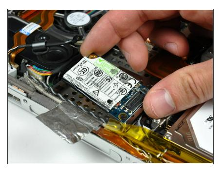
Lift the modem straight up off the studs on the PC card cage.
