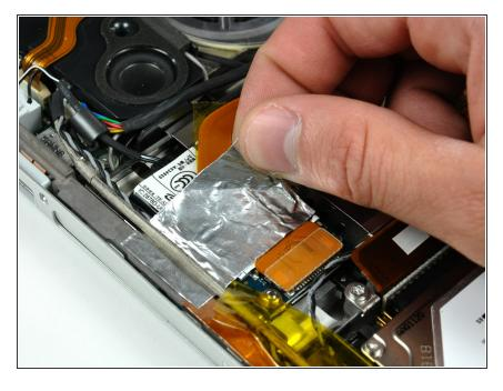
If necessary, peel back the strip of aluminum tape covering the modem cable.
