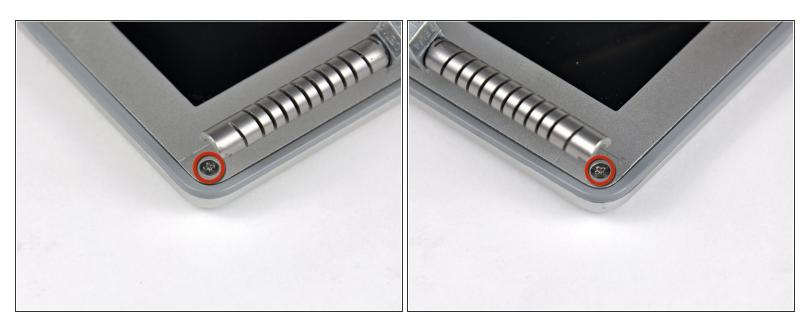
Remove the single Phillips screw from the lower left and right corners of the display.
