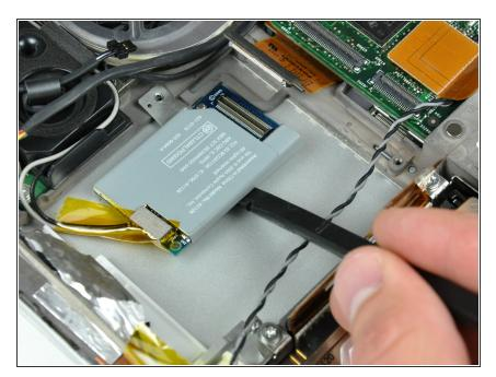
Use the flat end of a spudger to pry the AirPort/Bluetooth board up off the adhesive securing it to the lower case.
