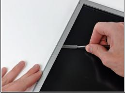
Continue running the edge of your metal spudger between the LCD frame and the front bezel until the right, bottom, and left sides of the LCD are free.
