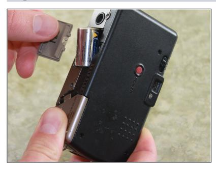
• Remove the battery from the camera by pulling the battery door outwards.
