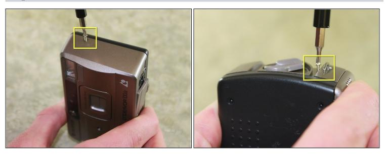
• Locate and remove the 6.4mm screws located on either side of the camera with a Phillips #00 screwdriver.
