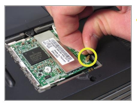
Disconnect the antenna cables from the Mini-PCI card.
