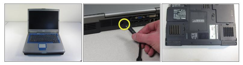
• Unplug the laptop from the power adapter and turn the power off.
