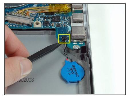
Disconnect the PRAM battery cable from the bottom right corner of the logic board.
