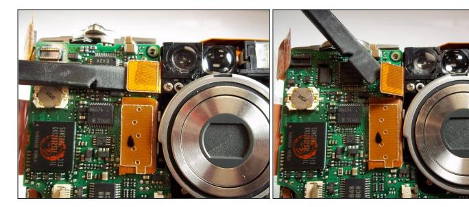
(i) Remove the next ribbon cable by using the flat end of the spudger to pry the cable from the board.
