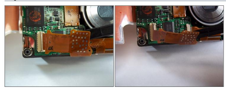
• Now, insert the spudger under the ribbon cable and gently pull the cable out of its port.
