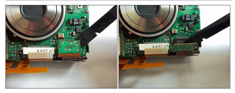
• The rest of the ribbon cables are not secured with ZIF connectors. Remove the ribbon cable on the bottom right corner of the motherboard by using the flat end of the spudger to pry the cable from the board.
