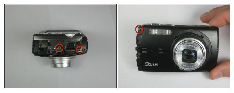
Remove the remaining three Phillips #00 side and front panel screws.
