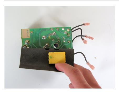
Gently peel back the protective film on the top of the transformer.
