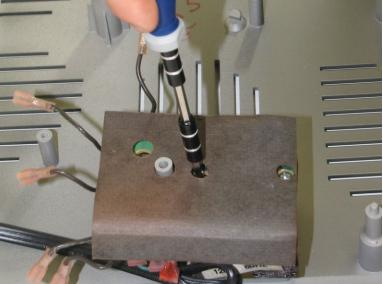
Remove the two 40.6mm Philips screws securing the TRS-80 transformer.
