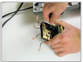
Remove the power cable jumpers from the power supply.
