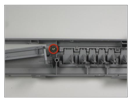
Remove the .384 inch screw holding the spring to front panel.
