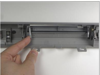
On back side of front panel very carefully apply pressure to the left hand side of the flap hinge.
