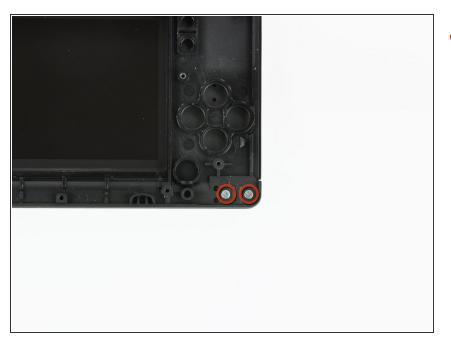
Remove the two 8.3 mm Phillips screws securing the upper case to the display assembly.
