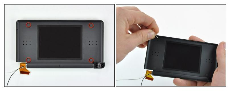
• Use a push pin to remove the four plastic screw covers on the front bezel.
