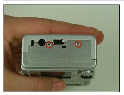
Remove the two 4.75mm screws located on the right side of the camera.(the side with the USB adaption plug)
