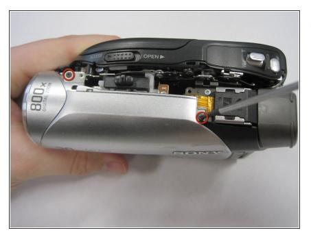
• Remove the two 2.9 mm screws under the black plastic casing.
