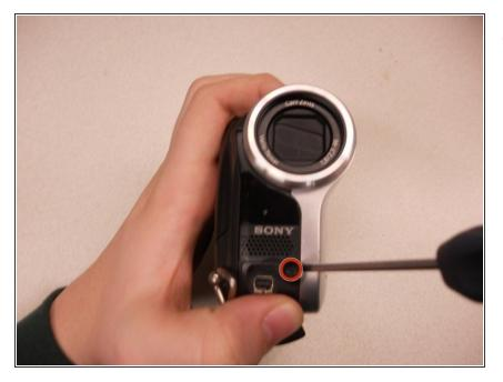
Remove the 4.5 mm screw under the output flap on the front of the camera below the lens.
