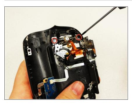
Remove (2) 5.4mm screws that are securing the screen to the cover, from the base of the LCD.
