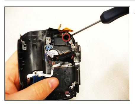
Remove (1) 2.9mm screw from the base of the LCD screen.
