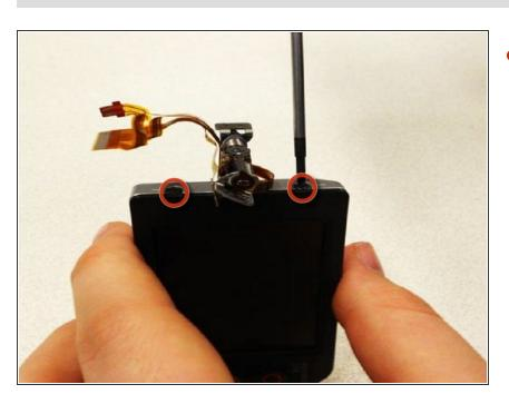
Remove (2) 3.8mm screws from the bottom of the LCD.
