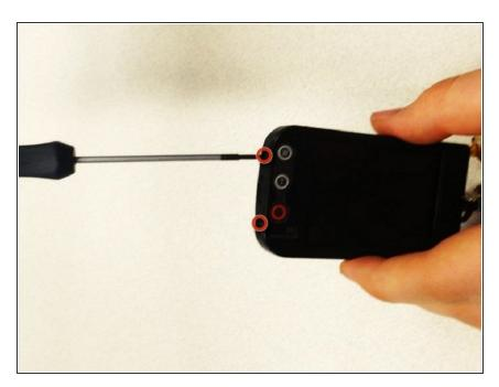
Remove (2) 3.8mm screws from the end of the LCD.
