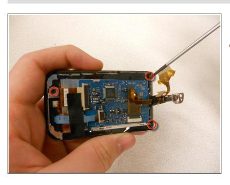
Remove (3) 4.5mm screws from back-side of the LCD.
