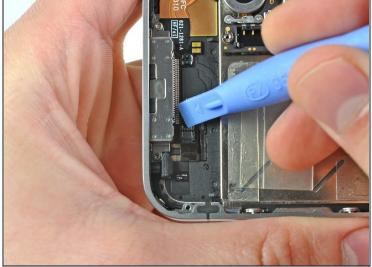
• Use a plastic opening tool to flip up the retaining flap on the home button ribbon cable ZIF socket.
