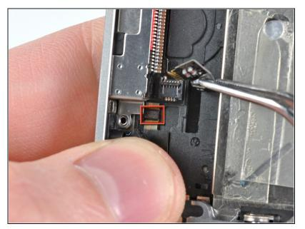
Remove the tiny rubber spacer near the dock connector.
