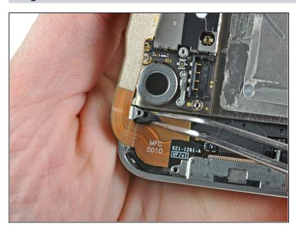
Use a pair of tweezers to remove the small rubber spacer beneath the speaker enclosure mounting ear near the vibrator.
