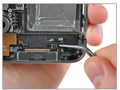
Use a pair of tweezers to pull the home button ribbon cable out of its socket.
