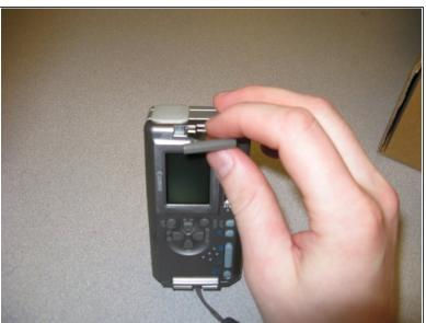
Remove the screen battery located to the left of the screen.
