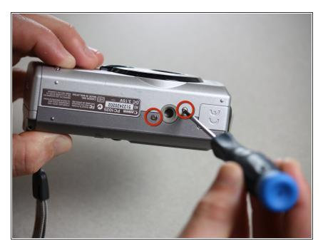
Use a Phillips #00 screwdriver to remove the two screws at the bottom of the camera.
