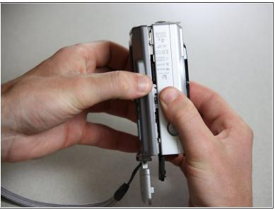
Carefully slide both halves of the camera together, making sure all tabs are aligned. Press the sides firmly together until you hear a click.
