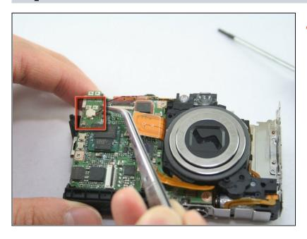
• Use the <u>tweezers</u> to disconnect the microphone cable.
