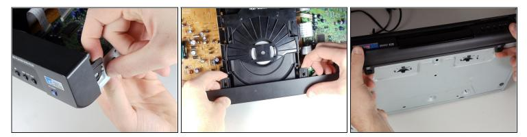
• There are six symmetrically placed tabs holding in the front faceplate. Unhook these six tabs to loosen the faceplate.
