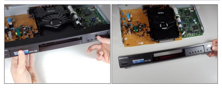
• Pull off front faceplate. This may take a couple of tries to get all six tabs unhooked simultaneously.
