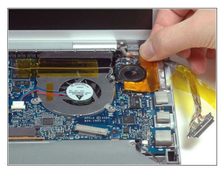
Peel up and remove the orange foil shield near the right speaker.
