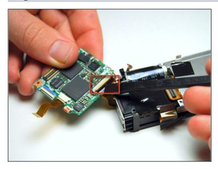
Use the spudger to open the black flip gate revealed under the motherboard. This gate attaches the copper ribbon to the motherboard.
