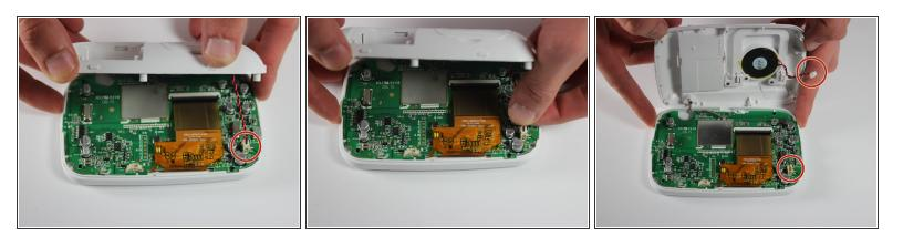
Disconnect speaker from monitor for ease of access by unplugging wire.
