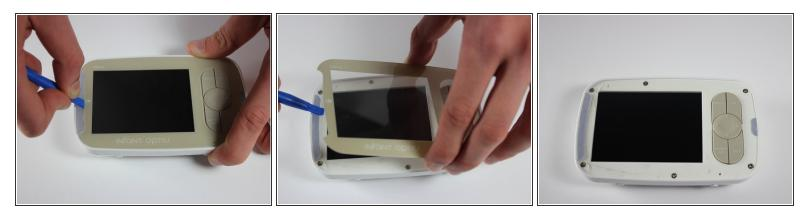
• Using the plastic opening tool, remove screen protector from front of monitor.
