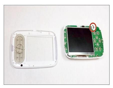
At the top right, the insulated wire exposes the antenna.
