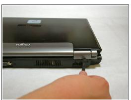
• Use a spudger to lift the back of the hinge cover on the left and right sides of the computer.
