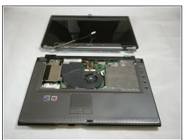
Hold down the body of the computer by placing your hands in the pictured positions. Then, lift the display from the body.
