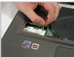
Unplug highlighted cables from the wireless module.
