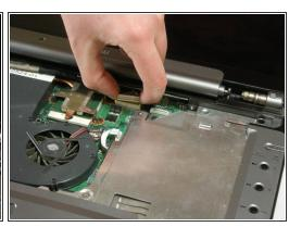
Use a spudger to detach and remove cables from the motherboard.
