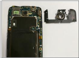
Remove the five 2.4mm screws located around the camera using a Philips head screwdriver to remove the plastic cover.
