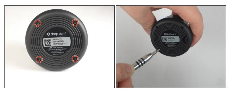
Using a Philips #0 screwdriver, remove the four 3 mm screws.
