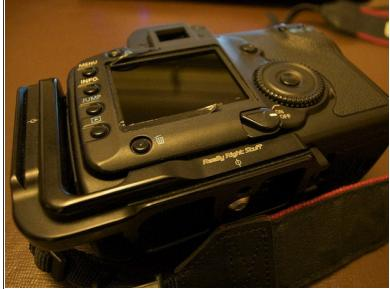
After removal, make sure to remove all pieces of the old lens. Checking for fragments of plastic, and dust on the LCD.
