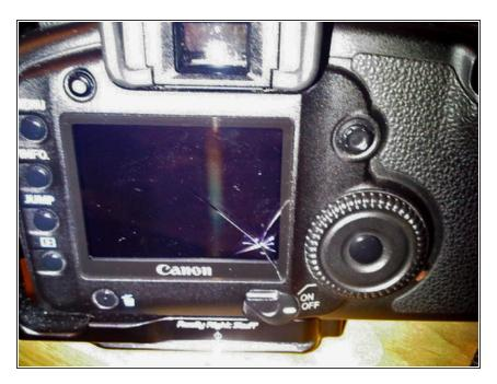
Here is the part we need to replace with a new LCD lens.
