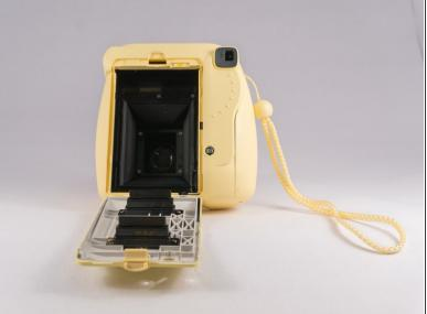
Open up the back and remove the film cartridge.
