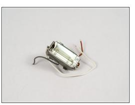
With a solder kit, heat the connecting solder points to open the connection, thus removing the connecting wires. There are many ways to do this, depending on the available tools on hand.
